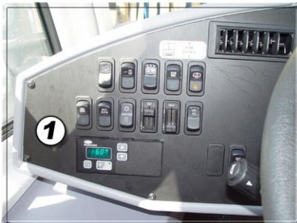
Figure 1 - Carrier control keypad and driver's controls
