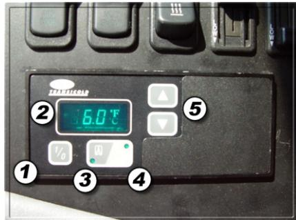
Figure 2 - Carrier keypad control functions
