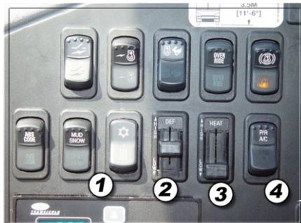
Figure 3 - Driver HVAC controls
